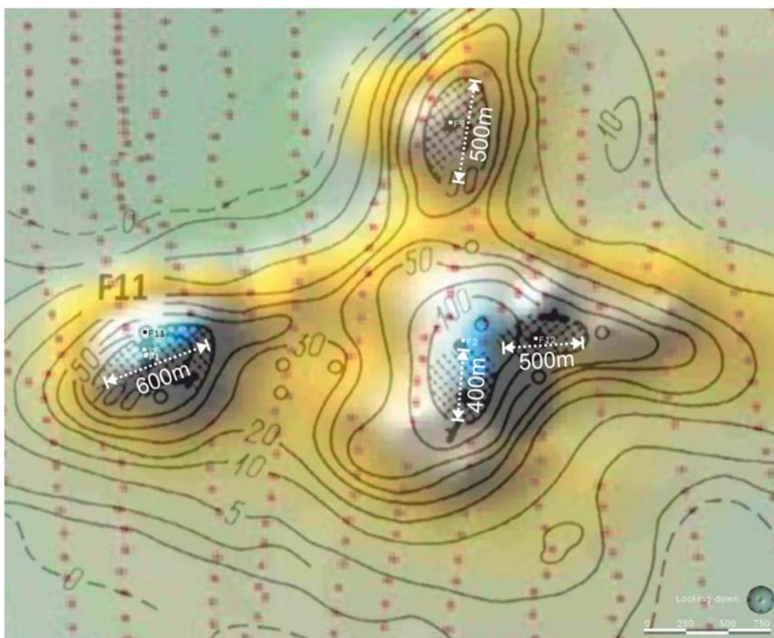
Figure 5-1: Estimated strike length of mineralised intersections
